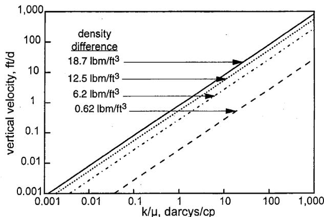
Fig. 12—Vertical velocity vs.  $k/\mu$  and density difference.
