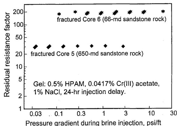
Fig. 11—Residual resistance factor vs. pressure gradient after gel placement.
