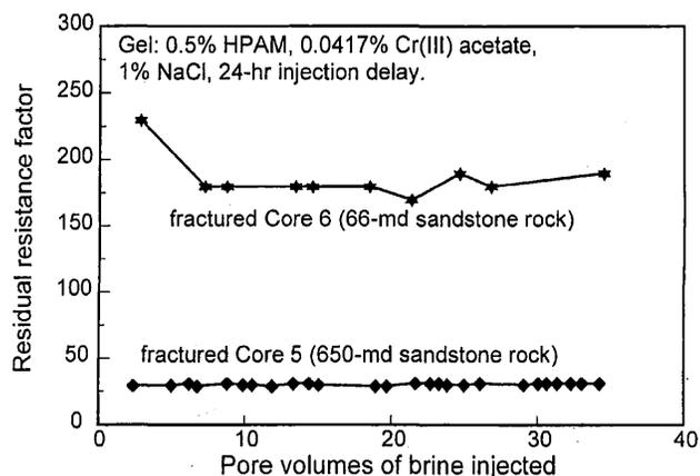
Fig. 10—Residual resistance factor vs. throughput after gel placement.
