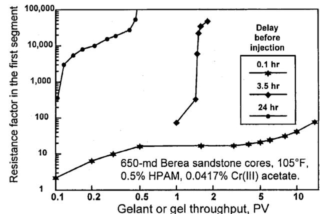
Fig. 3—Plugging in the first core segment for different delay times between gelant mixing and gelant injection.
