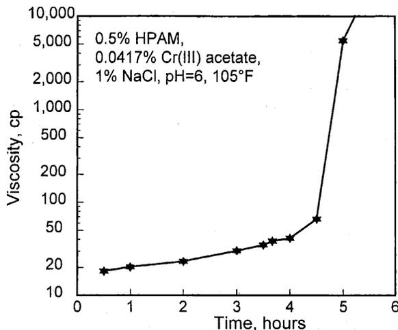
Fig. 2—Viscosity vs. time during gelation.
