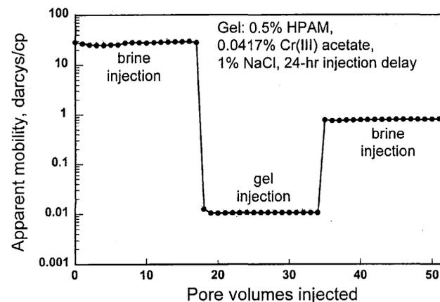
Fig. 7—Effect of brine and gel throughput on apparent mobility in fractured Core 7.
